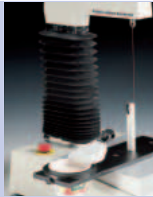
Small Peel Strength Rig (A/PS) Measurement of the peel strength of e.g. yoghurt containers – accommodates circular pots up to 80mm diameter
