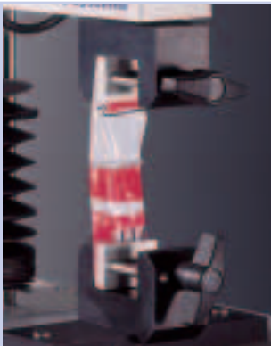
Tensile Grips (A/TG) Used for the assessment of Seal Strength
