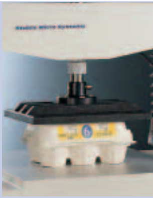
Compression Platen Used to assess packaging compressive strength
