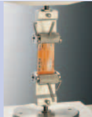
Self-tightening Roller Grips (A/TGT) Can be used to measure tensile strength of packaging where slippage at the grip face may be a problem
